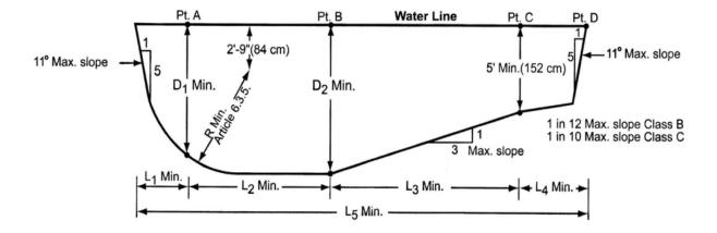
Figure 1 – Construction dimensions for water envelopes for Class B and Class C pools
